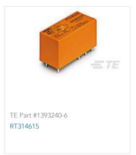
Force-Guided Relay, Monostable, 5A (NO) + 1B (NC), 8 A Contact Rating, 110 VDC Coil Voltage, 250 VAC Contact Voltage, 1.2 W Coil Power, SCHRACK SR6
