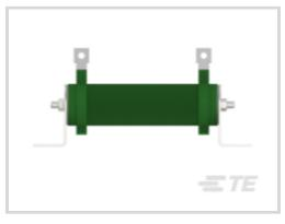
Resistor Type: Power Resistor Resistance Class: Up to  $1k\Omega$  Resistance Value: .47  $\Omega$  Power Rating: 50 W
