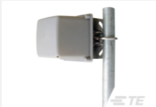
TE Part #MD24-12 Dir,Mini,Fixed,NF 2400-2485MHz, 11dBi,BW6
