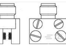
TE Part #1053478-1 SMA Stripline Launcher 2070 8002 92
