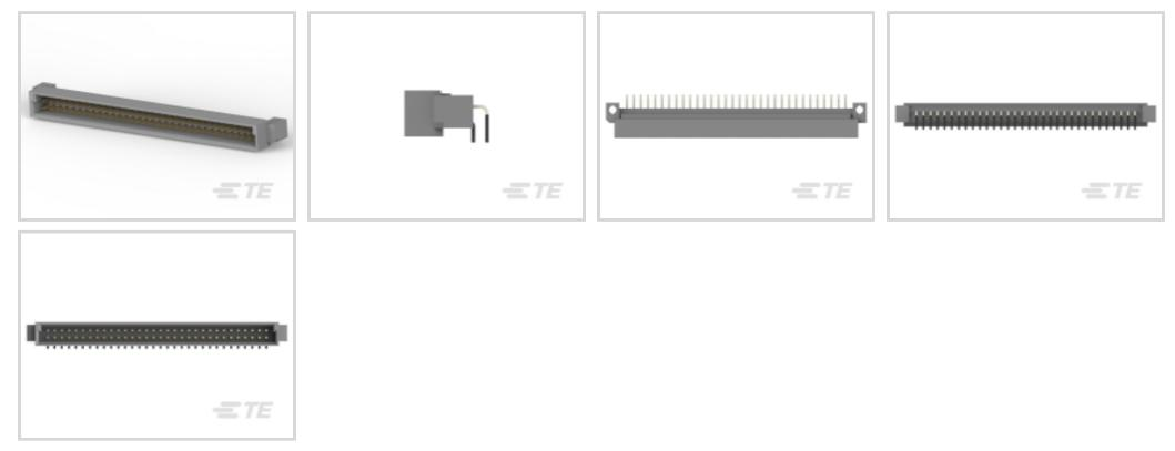
Connector & Housing Type: Plug Connector System: Board-to-Board Termination Post & Tail Length: 2.64 mm [.104 in ] Number of Positions: 64 Centerline (Pitch): 2.54 mm [.1 in ]
