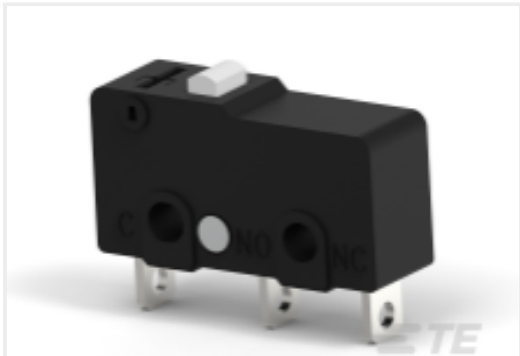
TE Part #2351450-1 SMINSA SW PPL 1.47N 5A/3A AC 3A DC SP
