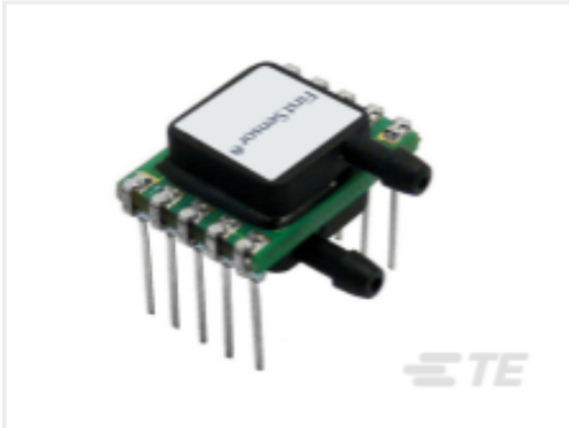
TE Part #1006943-F LDES500UF6S;PRES;0-500Pa;0,5-4,5V; 5Vs
