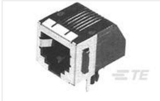
TE Part #5555140-4 MJ,LPF,R/A,6P/6C,SHLD,PNL GRD
