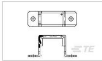
Terminal Junction Module Accessory Type: **Mounting Bracket**
