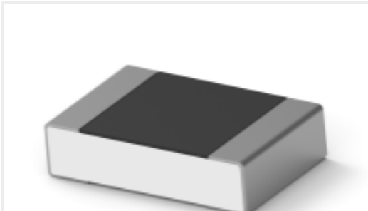
TE Part #5-2176378-8 RQ 0805 39R2 0.1% 10PPM 5K RL
