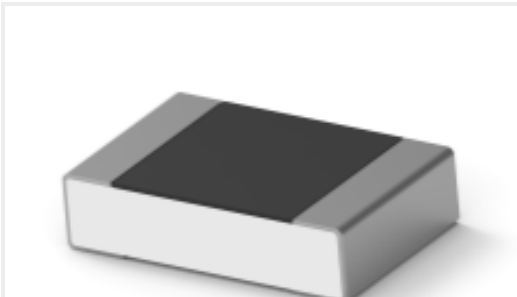
TE Part #5-2176378-6 RQ 0805 37R4 0.1% 10PPM 5K RL
