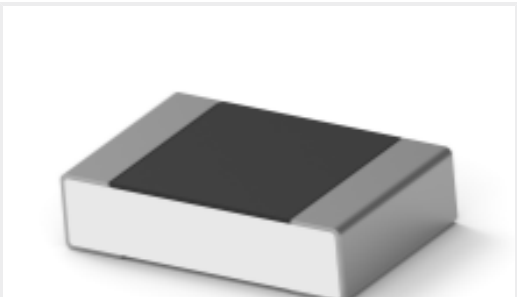
TE Part #5-2176378-9 RQ 0805 40R2 0.1% 10PPM 5K RL
