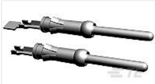
TE Part #1-66099-5 III+ PIN,18-16,TIN ,LP
