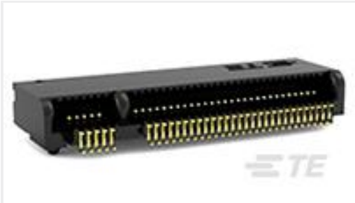
TE Part #2199119-6 M.2 0.5PITCH 3.2H KEY E 30U" AU
