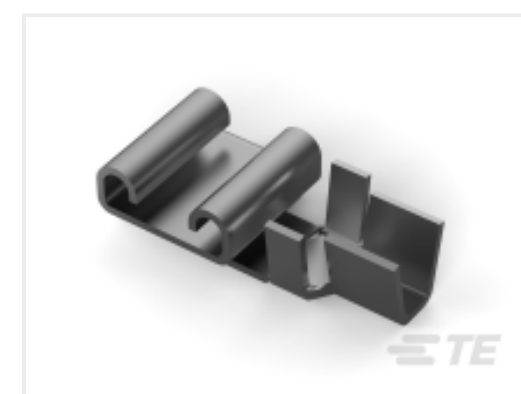
TE Part # 61188-1 250 FASTON FLAG REC 16-12 AWG TPBZ
