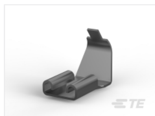
TE Part # 62057-5 250 FASTON FLAG REC 12-10 AWG TPBZ
