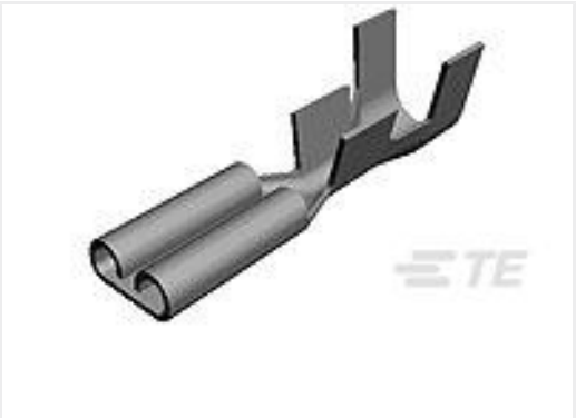
TE Part #160534-2 110 FASTON,REC.,17-20 AWG,TPBR
