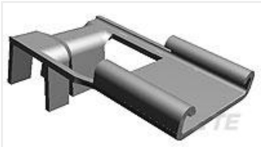
TE Part #60290-2 250 FASTON FLAG REC 18-14 AWG TPBR
