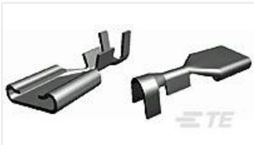
TE Part #42743-1 250 FASTON REC 22-18 AWG BR
