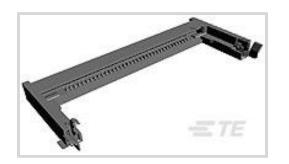
DRAM Type: Single Data Rate (M3) Connector System: Board-to-Board Number of Positions: 90 Termination Method to PCB: Surface Mount Module Orientation: Vertical
