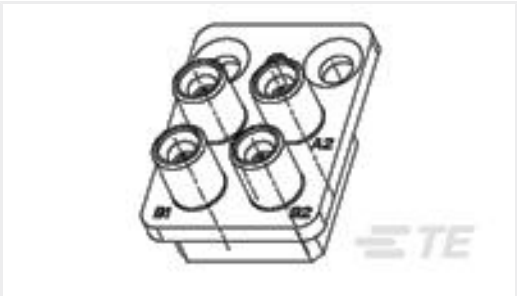
TE Part #1996884-1 4 Pos RF Module, Backplane,SMPM
