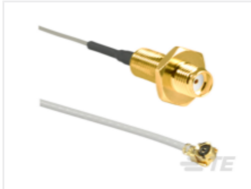
TE Part #CSI-SGFE-100-UFFR SMA to U.FL/MHF1 100mm 1.13 OD
