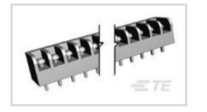
Number of Positions: 16 Barrier Strip Style: Tri-Barrier Bottom Termination Type: Printed Circuit Pin Connector System: Wire-to-Board Centerline (Pitch): 6.35 mm [.25 in ]
