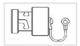
Data Bus Accessory Type: Dust Cap Data Bus Connector Style: Bayonet Polarization Code: D
