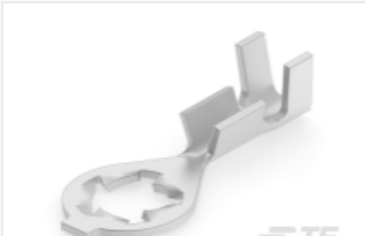
TE Part #2432197-2 RING, M4, DIA 4.3, 20-24 AWG, TPBR
