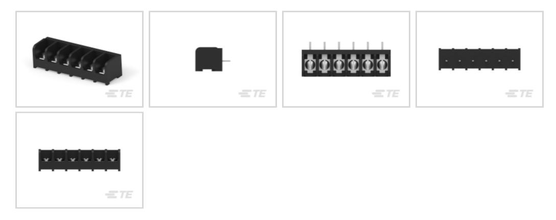
Number of Positions: 6 Barrier Strip Style: **Tri-Barrier** Bottom Termination Type: **Printed Circuit Pin** Connector System: **Wire-to-Board** Centerline (Pitch): **9.53 mm [.375 in ]**
