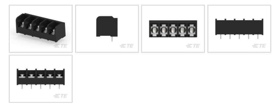
Number of Positions: 5 Barrier Strip Style: **Tri-Barrier** Bottom Termination Type: **Printed Circuit Pin** Connector System: **Wire-to-Board** Centerline (Pitch): **11.1 mm [ .438 in ]**
