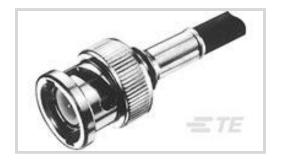
RF Interface: **BNC** RF Connector Style: **Plug** RF Connector Mated Outer Diameter (Approximate): **14.53 mm [.572 in ]** Impedance: **50 Ω** Compatible With RF Cable Type: **RG 174, RG 188**
