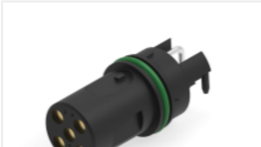
TE Part #225457-E M12 FEMALE, A CODE,RA, 5P THR REAR MOUNT
