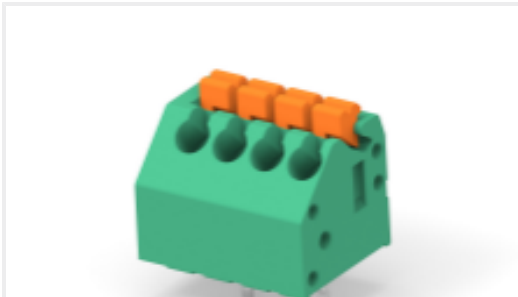
TE Part #1-2834011-4 4POS 3.5MM TOP ENTRY SCREWLESS CONN.
