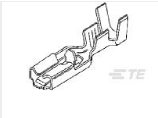
TE Part #63520-1 PL 187 TERMINAL REC 20-16 AWG TPBR
