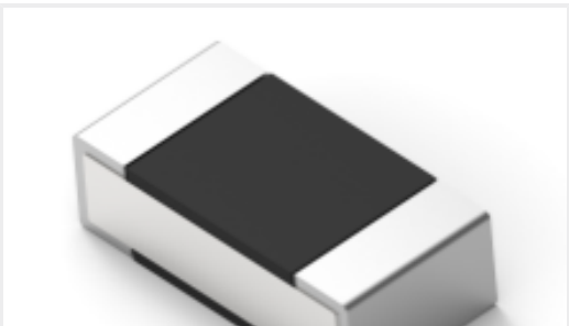
TE Part #9-2176305-7 RP 1E 0.1W 1K07 0.1% 25PPM 5K RL
