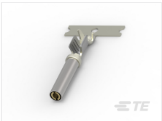
TE Part #2098251-1 SOC, SF, SIZE 16, 16-18 AWG, AU/SN
