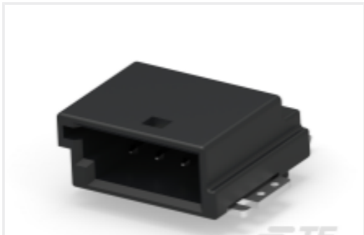
TE Part #967688-3 4pos MQS .63 header 90deg SMD
