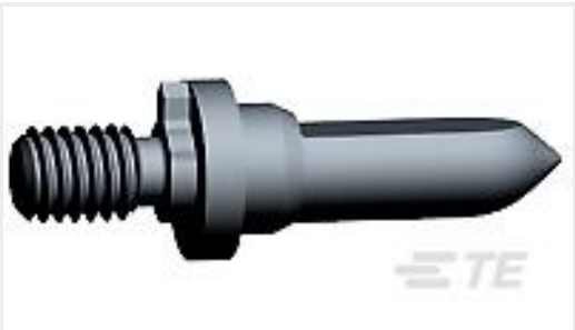
TE Part #2000676-5 Keyed Guide Pin, Machined, Vita 46
