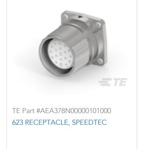
Cable-to-Panel, Power, Panel Mount, Electrodeposited Nickel, Zinc Alloy, PA66, 40 Shell Size, Shielded, Metal, -20 – 130 °C [-4 – 266 °F]
