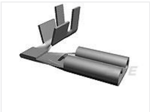
TE Part #62336-1 110 FASTON FLAG REC 22-18 AWG TPBR
