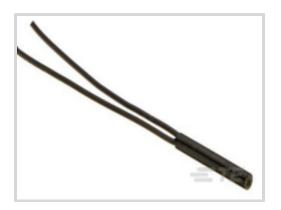
NTC Sensor Type: NTC Thermistor Lead Wire Length: 56 mm [2.205 in]Resistance (at 25°C):  $10 \text{ k}\Omega$ Resistance Tolerance (at 25°C):  $\pm .88 \%$ Tolerance  $\beta$ -Value:  $\pm .5 \%$
