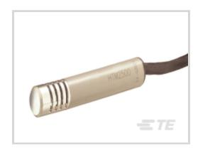
Operating Temperature Range: -40 – 85 °C [-40 – 185 °F] Humidity Sensor Product Type: RHT Module Supply Voltage (Peak): 12 VDC Accuracy: ±3 %RH Nominal Output @55%RH (at 5 VDC): 2.48 V
