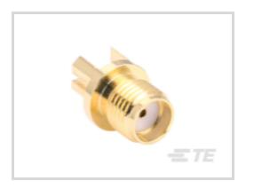
RF Interface: SMA RF Connector Style: Jack Impedance: 50 Ω RF Connector Coupling Mechanism: Threaded Operating Frequency: 0–18 GHz
