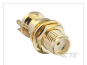
TE Part # L9000272-01 SMA Jack 50 Ohm .062 PCB Edge Mount
