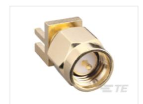
TE Part #L9000276-01 SMA Plug 50 Ohm .062 PCB Edge Mount
