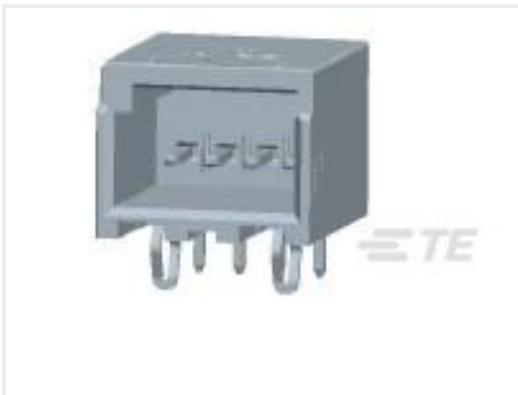
TE Part #1-1939761-4 HDR ASSY (H-TYPE) 4POS X-KEY TIN
