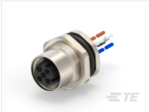
TE Part # T4171110505-802 M12,REAR MOUNT,FEMALE,D,5P,0.5 M WIRE
