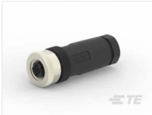
TE Part # T4110502051-000 M12,FEMALE,STRAIGHT,D CODE,5P, PG9,GOLD
