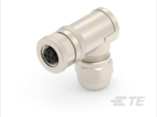
TE Part #T4112511051-000 M12 F, 5P GOLD D_CODE RA SHIELDED PG7
