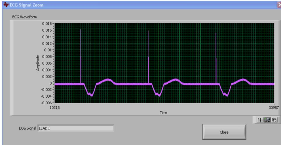
Figure 35. Digitization of PACE Signal Using ADS1298
