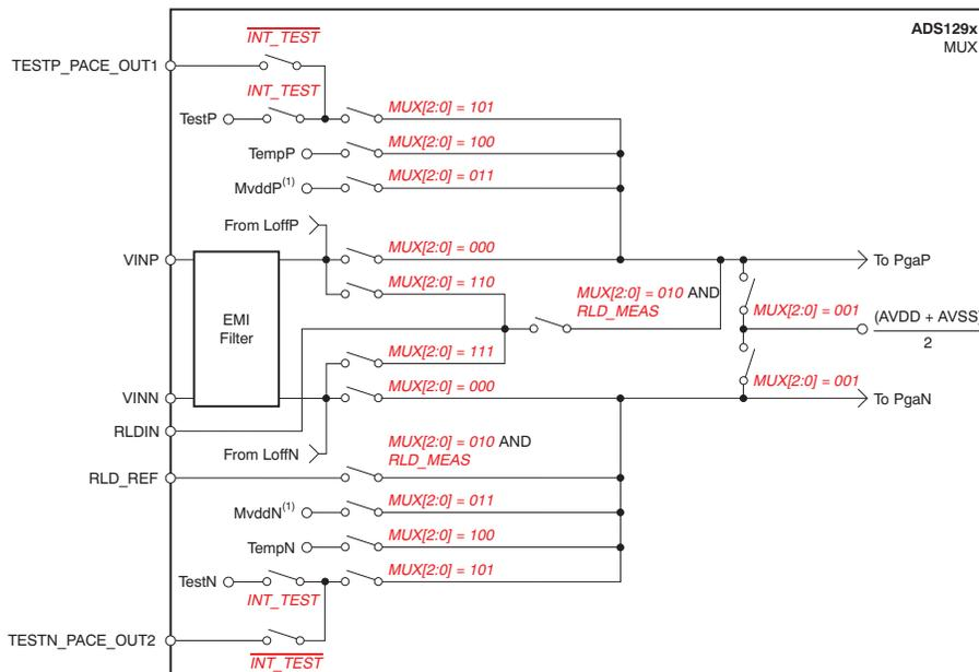
Figure 11. Input Multiplexer for a Single Channel
