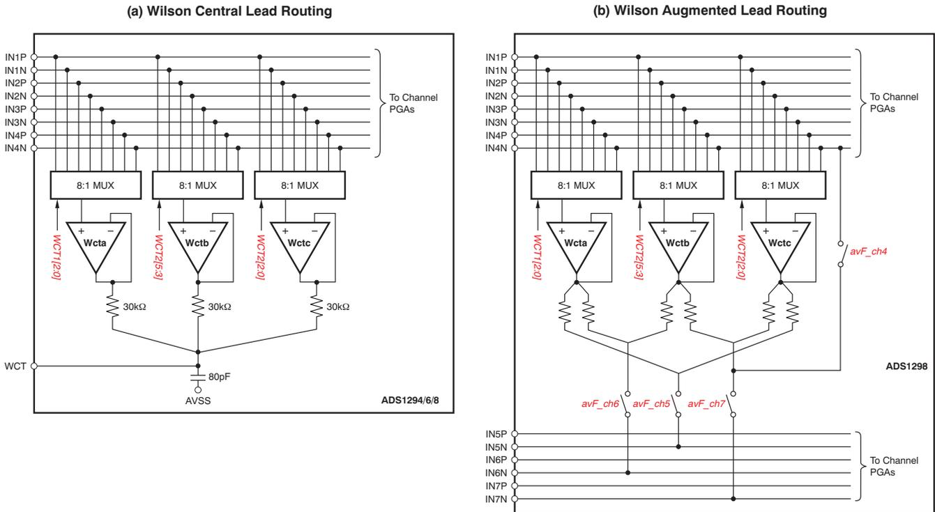
Figure 15. Wilson Central and Augmented Lead Routing Diagrams
