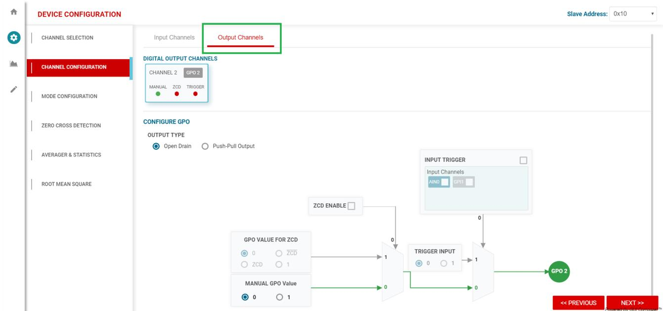
Figure 13. Channel Configuration Page, Output Channels Tab
