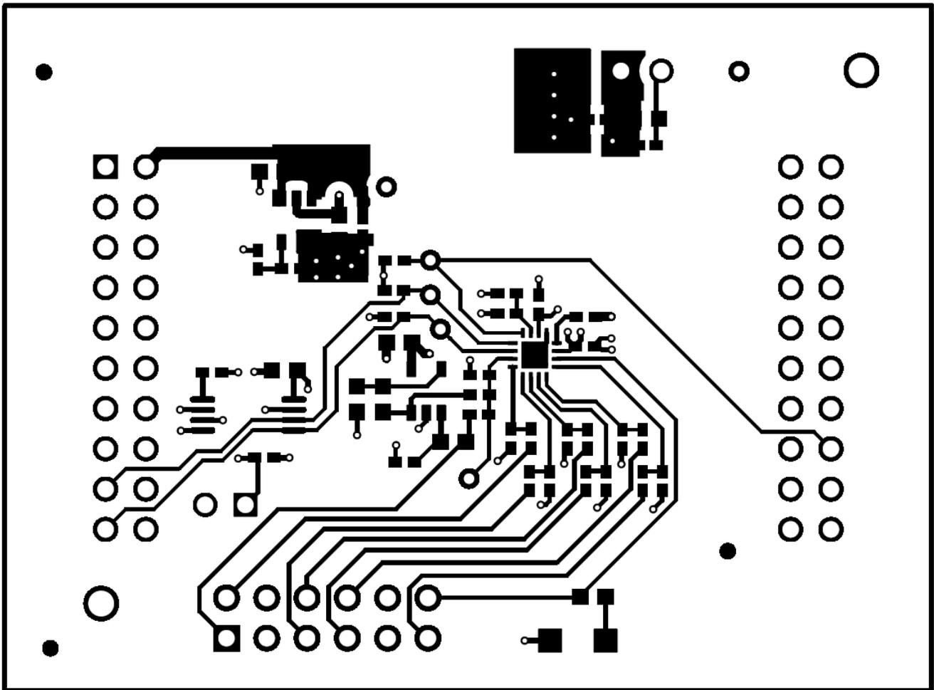
Figure 27. BP-ADS7128 Top Layer Copper and Silkscreen
