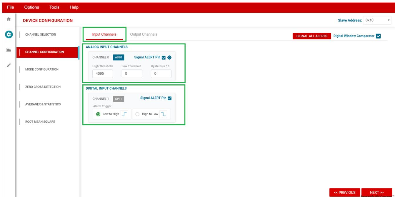
Figure 12. Channel Configuration Page, Input Channel Tab
