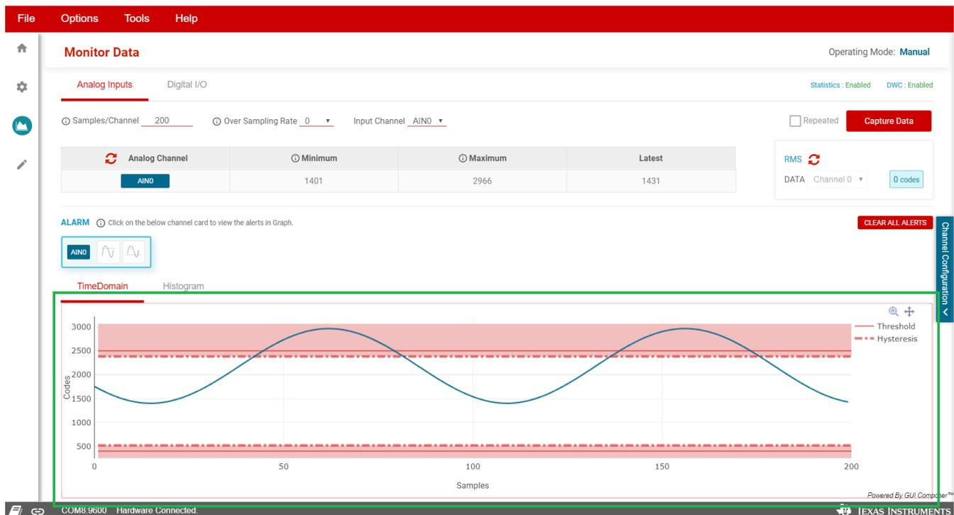
Figure 22. Time Domain Display With Threshold and Hysteresis
