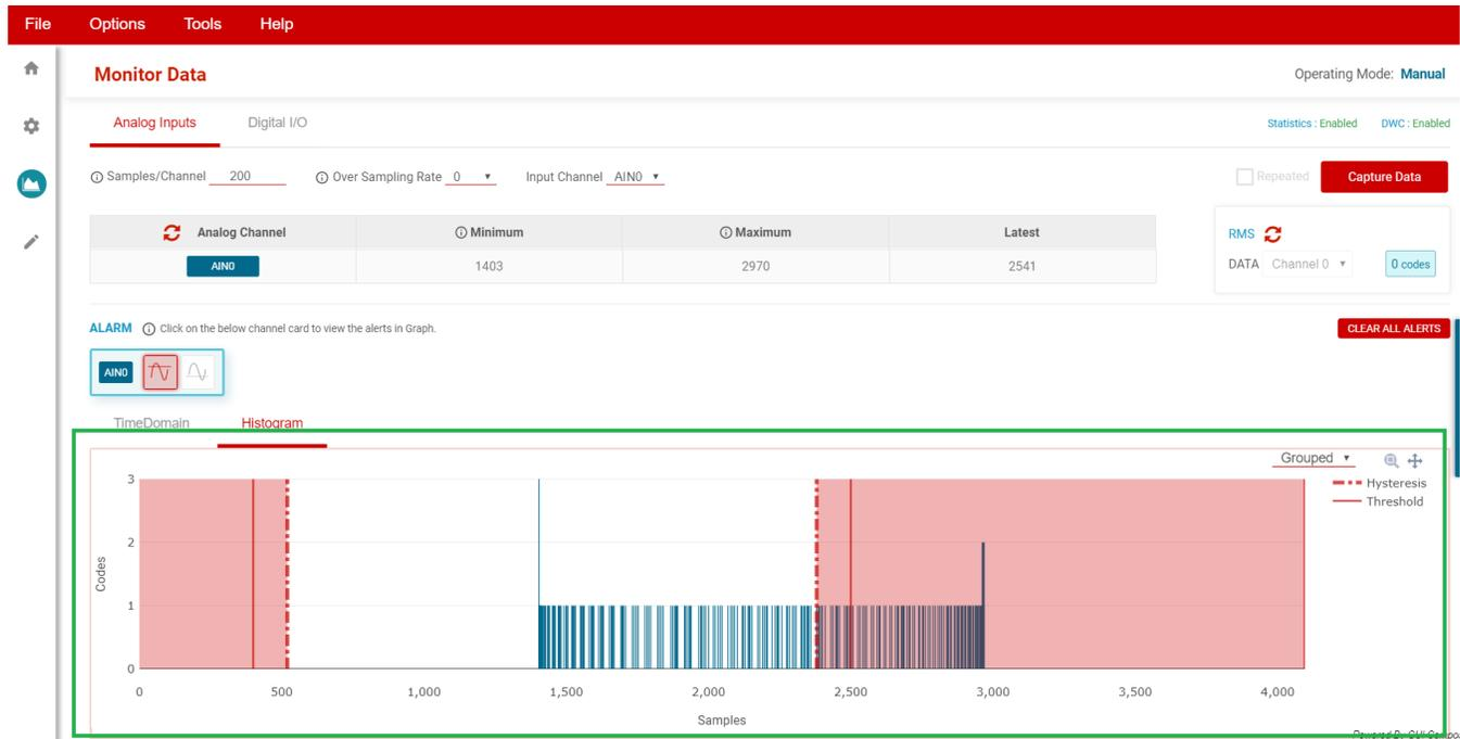
Figure 23. Histogram Graph Display With Threshold and Hysteresis
