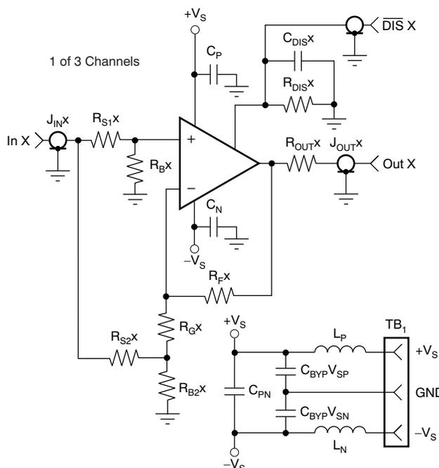
**Figure 2. Schematic for DEM-OPA-SSOP-3B**
