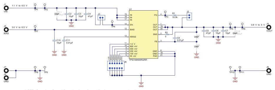
NOTE: Capacitors C1 and C8 and resistors R3 and R4 do not come populated.
