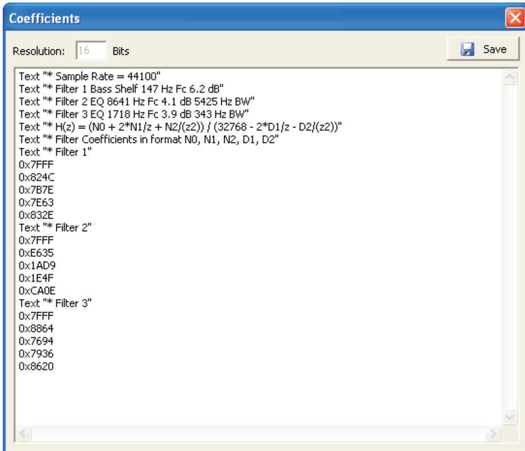
**Figure 6. Filter Coefficients**
