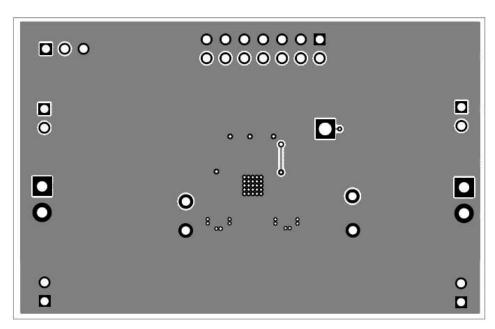
Figure 5. Bottom Layer Routing
