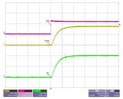
NOTE: C1 (yellow) VOUT - Turnon Ramp to 1.8V, C2 (red)  $I_{IN}$  – Surge Current for a Fully Loaded output.
