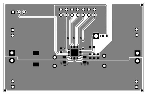
Figure 4. Top Layer Routing
