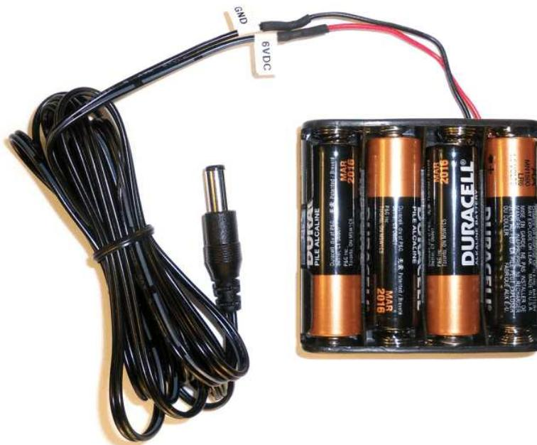
Figure 69. Recommended Power Supply for ADS1299EEG-FE
