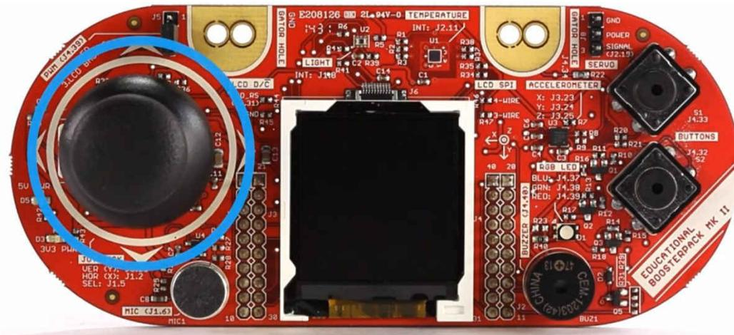
**Figure 3-2. 2-Axis Analog Joystick With Digital Input**
