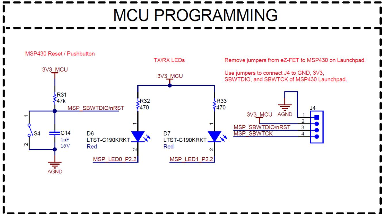
Figure 8-3. MCU Programming and Debug Schematic
