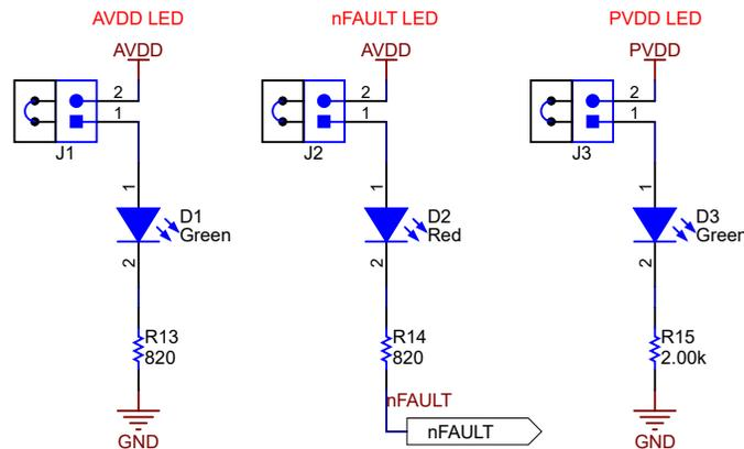
Figure 8-6. Status LEDs Schematic
