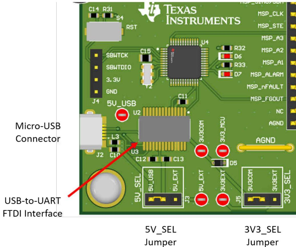
Figure 4-3. Micro-USB Connector and UART for MCT8329EVM
