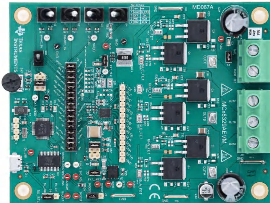
Figure 2-1. MCT8329EVM Printed Circuit Board (PCB - Top View)
