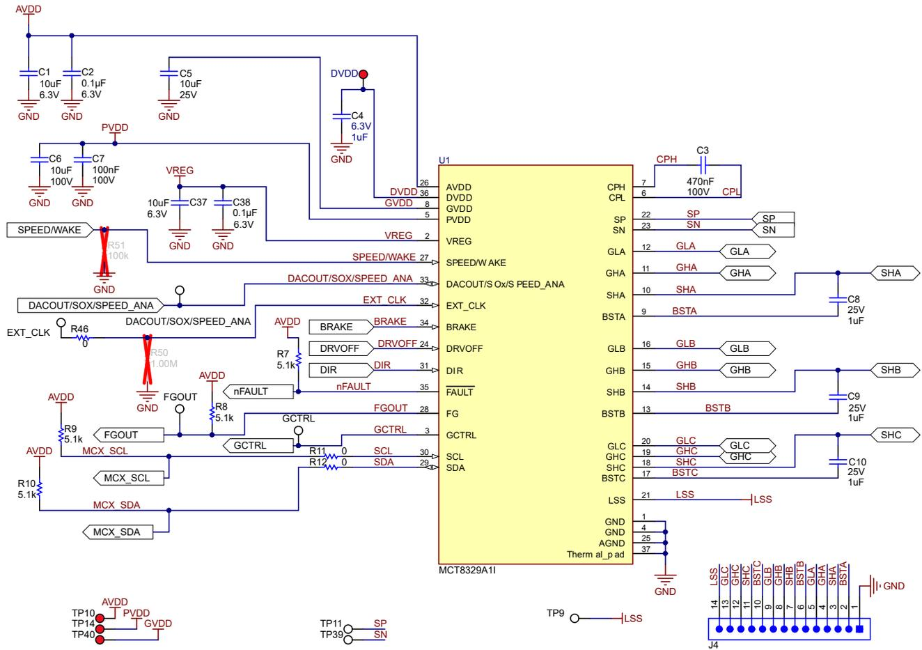
Figure 8-5. MCT8329A 3-Phase Sensorless Trapezoidal Gate Driver Schematic
